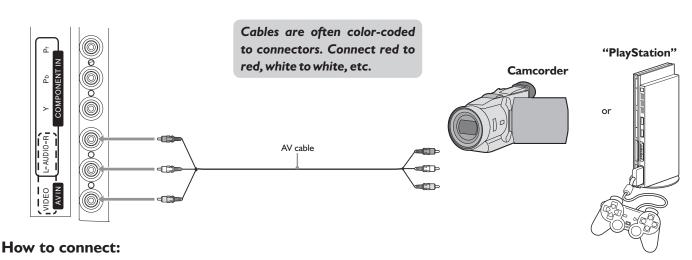
Connect the Audio/Video cables between the Audio (L/R)/Video jacks on the unit and camcorder.
